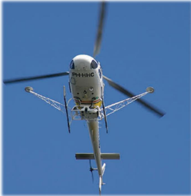
Aerial LiDAR Survey at 40 scans per metre
